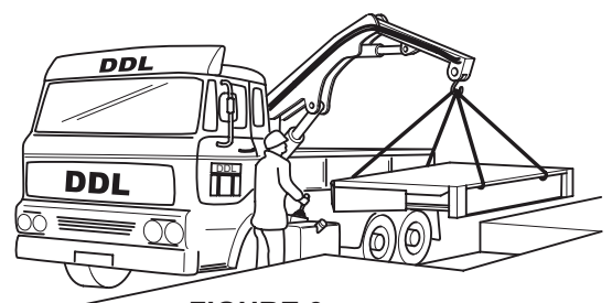
FIGURE 3c Via Mobile Crane
