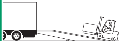
MOBILE RAMP REQUIRES ADDITIONAL YARD SPACE AND HIGH GRADABILITY LIFT TRUCK 1 Man + Ramp @ 1 ¼ Hours = 1 ¼ Man Hours
