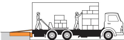
PALLETISING ON VEHICLE OR CONTAINER FLOOR 2 Man @ ¼ Hour = 1 ½ Man Hours
